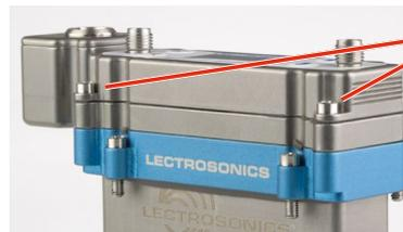
Slide the adapter up and tighten the retaining screws to secure it to the receiver flange.
