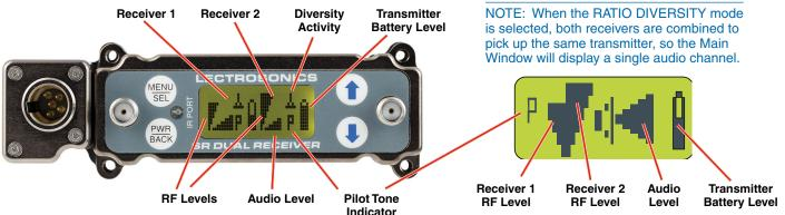
The Main Window displays information concerning the condition of the Pilot Tone, antenna phase, RF and audio signal levels and battery conditions for both the receiver and the associated transmitter.
