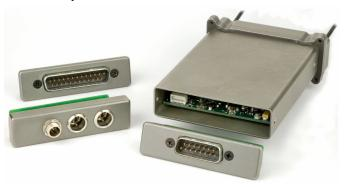
Power and audio connections are made through mating connectors on the adapter and receiver main circuit boards.
