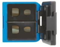
A pressure plate on the battery door compresses the battery contacts to maintain a solid connection with the batteries.
