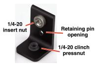
The bracket provides two different mounting nuts. The standard pressnut is used to attach the sleeve. The tensioning (clinch type) pressnut is used to attach the cold shoe mounting foot. Attach the bracket to the sleeve with the long pan head screw into the standard pressnut. The retaining pin fits into the opening in the bracket. Attach the cold shoe mounting foot to the tensioning nut and rotate it to orient the receiver as desired.
