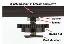
For horizontal mounting, insert the cold shoe foot into the clinch nut in the sleeve. Rotate the foot to the desired postion, then tighten the jam nut to lock it in place.
