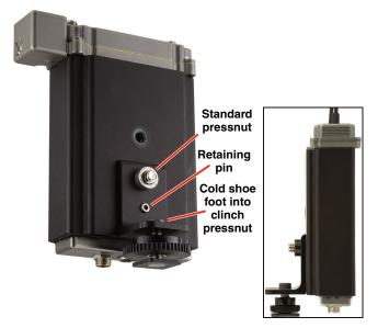
The clinch nuts in the foot and housing apply friction to the threads to allow the foot to be rotated to the desired position, with the jam nut locking it in place. Use a wrench to rotate the foot, then tighten the jam nut to prevent the foot from rotating.
