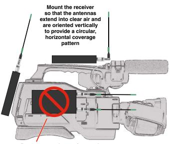
Do not mount the receiver so the antennas will be next to another piece of equipment nor oriented horizontally
