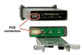
Slide the battery sled adapter into the end of the SR and gently seat it into place with the rear panel flush with the housing.
