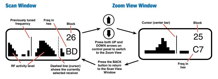
Spectrum scanning with the receiver itself is the best way to find clear operating frequencies, since it will reveal all RF signals present in the receiver, including those generated by IM (intermodulation).
