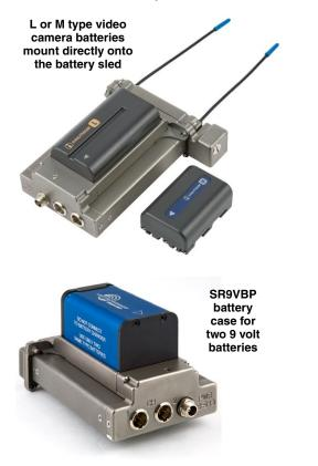
The battery sled adapters do not include charging circuitry. Batteries must be charged with their respective chargers. The adapters include an integral circuit that automatically selects between the battery and the external source, whichever delivers the highest voltage.
