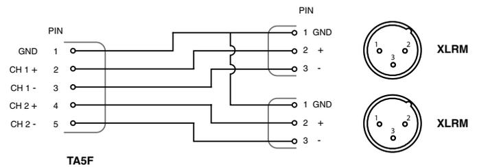
Right angle TA5F plug (RATPAC connector) to two 3-pin XLR; balanced outputs; 20 inches long.
