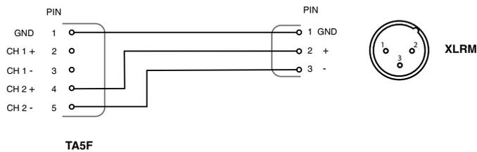
Right angle TA5F plug (RATPAC connector) to one 3-pin XLR; balanced output; 20 inches long.
