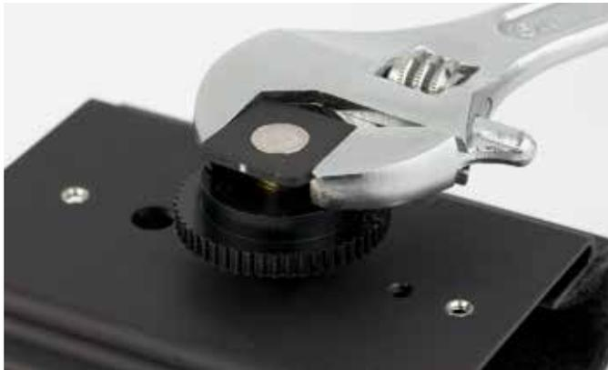
2. Use a wrench to thread the stud in about 1 - 2 turns, then rotate it to orient the receiver control panel in the desired direction.
