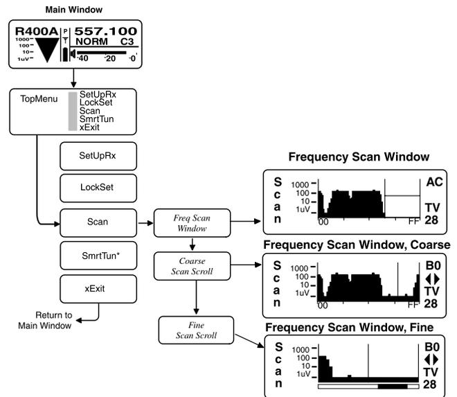
the tuning range. As the cursor scrolls across the frequency band, Frequency Select Switch settings for the associated transmitter are shown in the upper right corner of the screen.
