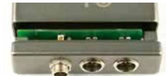
Align the mating connectors and slide the panel straight into the housing until the screw holes align with the housing.
