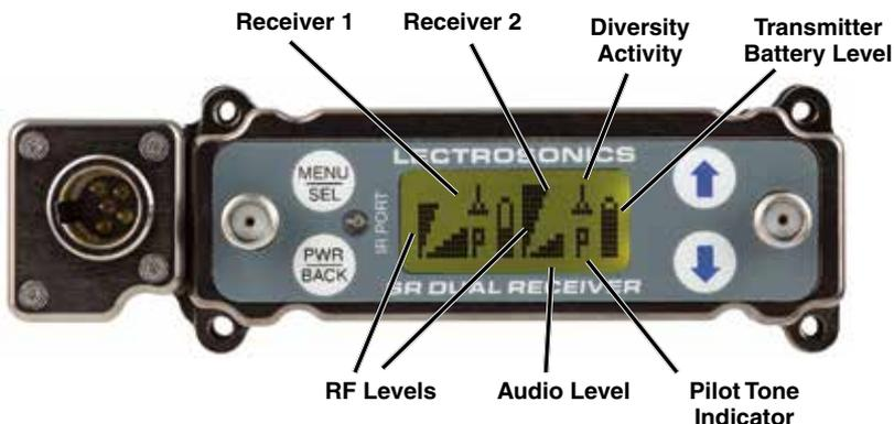
The Main Window displays information concerning the condition of the Pilot Tone, antenna phase, RF and audio signal levels and battery conditions for both the receiver and the associated transmitter.
