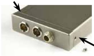
Panels are held in place by two Phillips head screws on the sides of the housing.
