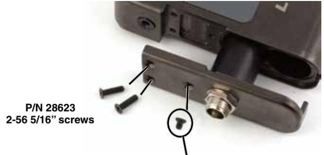
**CAUTION:** Use only the shorter screw P/N 28615 2-56 1/8" in the hole near the connector. The longer screws may damage a circuit board component.
