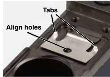
Place the spring detent clip on the housing with the tabs facing upward and the screw hole aligned with the one in the housing.
