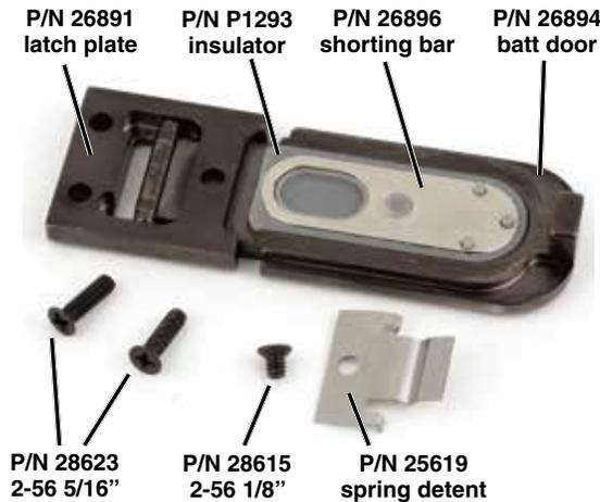
Assemble the battery door and latch plate.
