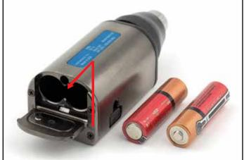
Slide the battery door outward, then swing it open. Batteries operate in series, with a connecting plate built into the battery door.
