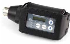
Clear plastic window allows access to the control panel
