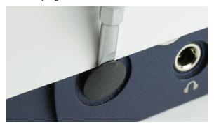
Insert the straight end of the coaxial cable through the hole in the front panel.
