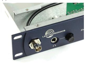
Antennas can still be connected to the rear panel by simply disconnecting the internal cable at the rear panel BNC connector.
