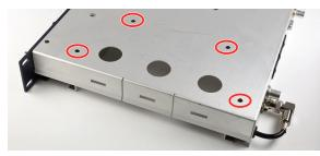
Route the coaxial cable along the side of the module compartment and fasten it to the tabs on the compartment housing with the tie-wraps.
