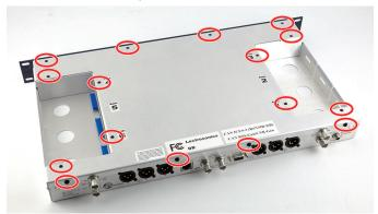
Turn the receiver over and remove the four screws that hold the module compartment housing. The shield cannot be removed, but it will move enough to allow better access to the front panel hole plug and cable routing.
