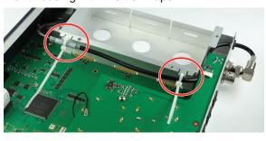
Trim off the excess end of the tie-wraps and bend the tab on the compartment housing down slightly to allow clearance for the cover.
