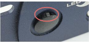
Use a small, flat blade screwdriver to press downward on the retaining tabs. Place a piece of thick paper (card stock) between the screwdriver and the panel to avoid scratching the finish, and pry outward to remove the hole plug.
