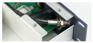
Rotate the cable to align the flat in the threads with the flat in the hole so the connector is fully seated, then tighten the nut to hold the connector in place. *Tighten the nut gently* with an adjustable ("crescent") wrench.
