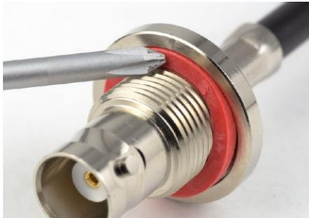
1. Begin by removing the flat nut, red sealing washer and locking ring (under red sealing washer) from both cables.
