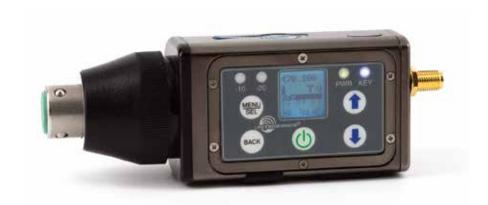
WARNING: Moisture, including talent's sweat, will damage the transmitter. Wrap the DPR-A in a plastic baggie or other protection to avoid damage.
