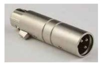
This polarity reversing adapter may be needed to correct for asymmetrical current draw in some P48 powered condenser microphones, including older Neumann 100 Series, Rode NTG3 and others. If your microphone does not power on correctly when used with these transmitters, insert the adapter between the transmitter and microphone.
