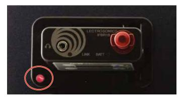
When a battery or IFBR1B is being charged the LED next to it will glow RED. When the battery is fully charged, the LED will glow GREEN.
