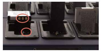
OR up to four IFBR1Bs (or a combination of each). You will know that your connection is correct on either a battery or IFBR1B when the LED illuminates.
