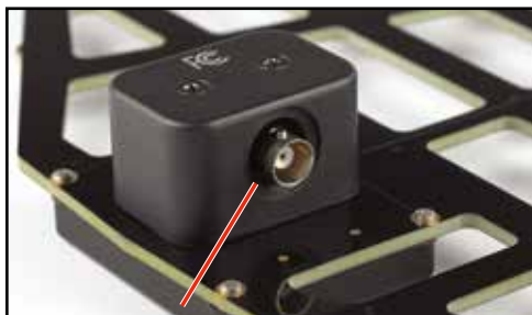
Power is provided by DC bias on the output connector
