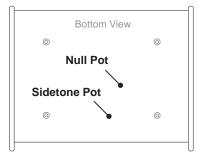
while wearing a broadcast headset, or separate headphones and microphones. Ideally, this adjustment is made with two people on headsets, after setting mic and headphone levels for broadcast. To adjust intentional sidetone level, insert a small flat blade screwdriver into the Sidetone level trim pot and adjust to desired level. Replace the hold plug when finished.
