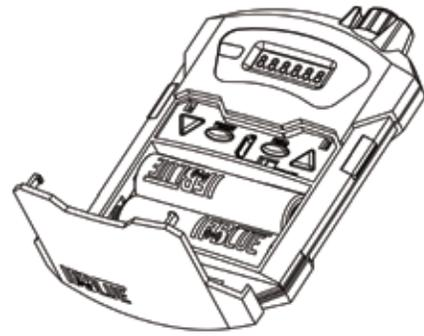
IFBR1C functions with two (2) AA batteries (+1.5 VDC each); alkaline, lithium, or NiMH rechargeables (supplied). Pinch the buttons on each side of the battery door, and pull the door toward you to open. Install the batteries according to the polarity diagram. Select either “primary” (non-rechargeable) or “NiMH” (rechargeable) via the slide switch next to the USB connector. Press the battery door closed until you hear the retaining clasps snap.
