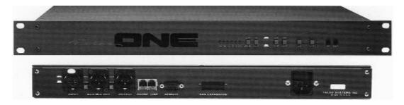
The Telos ONE input may be switched to accommodate either mic or line level. Two outputs are provided, one of which may be switched to provide either an independent caller output or a mix of the input and caller signals. Modular jacks are used for connection of the phone line and, if desired, a
