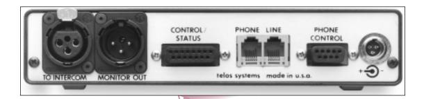
The intercom buss is connected to the TO INTERCOM XLR on the Link rear panel. The MONITOR OUT provides a convenient way to listen to both sides of the conversation. Phone line and set connections are via standard modular jacks. The DB-9 and DB-15 connectors offer full remote and status capability and provide four-wire inputs and outputs.
