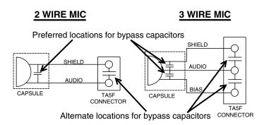
capacitors can be installed on the mic wires inside the TA5F connector housing.
