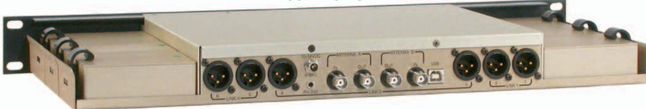
The rear panel provides six balanced audio outputs on standard XLR connectors, 50 ohm BNC antenna inputs, 50 ohm BNC antenna outputs from the built in zero-gain multicoupler, power jack with a locking connector, USB port and RS-232 serial port for the computer interface.
