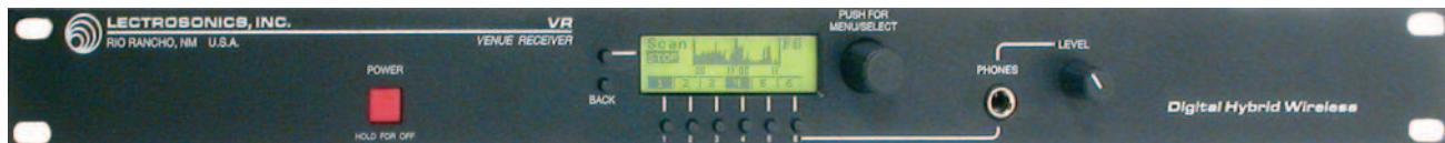
The front panel provides an easy-to-use LCD interface for setup, and provisions for quick monitoring to assist in troubleshooting. In normal operation, the LCD shows RF and audio levels, diversity status, pilot tone status (where applicable) and transmitter battery status (when available)
