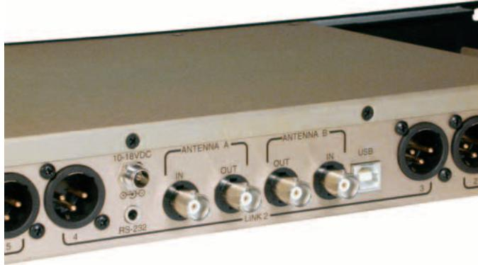
50 Ohm BNC multicoupler output jacks provide zero-gain antenna "loop-throughs" for an additional receiver, allowing convenient expansion without the need for an external RF multi-coupler.
