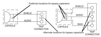
Install the capacitors as follows: Use 330 pF capacitors. Capacitors are available from Lectrosonics. Please specify the part number for the desired lead style.
