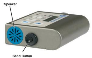
When the transmitter is in the power saving sleep mode, it uses only 20% of the normal battery drain, so battery life with be 5 times longer. This is especially useful in situations where the transmitter is buried deep inside costuming and there are waiting periods between use. The transmitter can "sleep" for several hours and then be awakened and adjusted when the production is about to begin.
