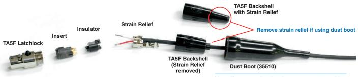
Note: If you use the dust boot, remove the rubber strain relief that is attached to the TA5F cap, or the boot will not fit over the assembly.
