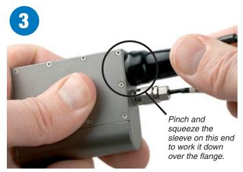
Squeeze the end of the sleeve so you can feel the connector inside and press it into the jack until it latches. Pinch and squeeze the sleeve near the flange and work it down with a kneading motion over the flange all the way around until it stays in place flush with the housing. Pull on the connector to make sure it is firmly latched.
