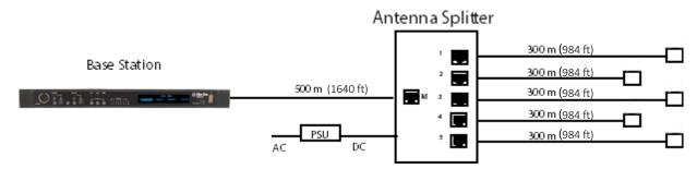
Figure 3-1 Recommended antenna and splitter powering schemes and cable lengths, PSU at splitter only
