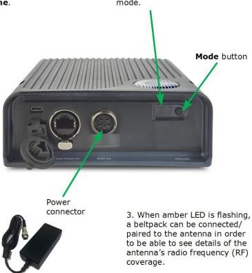
Figure 3-6 Using an antenna and beltpack in standalone mode
