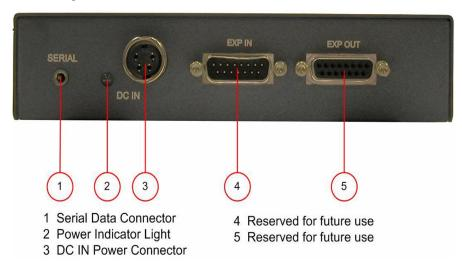
Figure 9-4 FS II Splitter Rear Connector Panel
