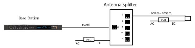
Figure 4-8 Recommended splitter and antenna powering schemes and cable lengths, PSU at splitter and antenna/transceiver
