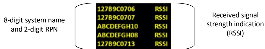
Figure 3-4 An unconnected beltpack site survey screen
