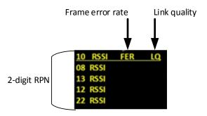
Figure 3-4 A connected beltpack site survey screen
