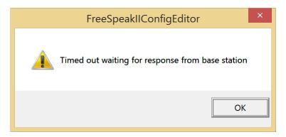
Figure 10-5 Configuration Editor Ethernet Timeout
