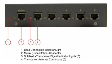
Figure 9-3 FS II Splitter Front Connector Panel
