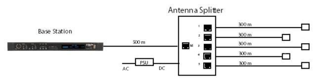
Figure 4-7 Recommended antenna and splitter powering schemes and cable lengths, PSU at splitter only
