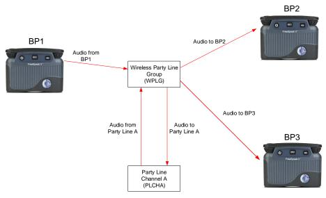
Figure 4-5 Connecting beltpacks to a wired partyline
