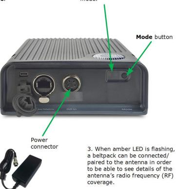
Figure 3-6 Using an antenna and beltpack in standalone mode
