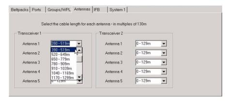
Figure 10-20 Antenna Cable Length Setup
