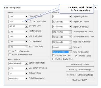
Figure 10-12 Set beltpack master volume low level limiter
