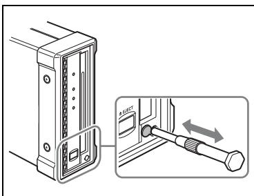
After ejecting the disc, it is not necessary to return the lever to its original position. The next time the unit is powered on, normal operation will resume.
