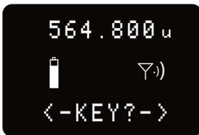
The DSSM ships with the key type set as “Universal” and will work right away with any receiver also set to Universal Key Type.
