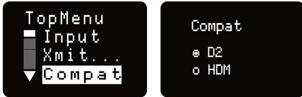
Use the **UP** and **DOWN** arrow buttons to select the desired mode, then press the **BACK** button twice to return to the Main Window. Compatibility modes are as follows:
