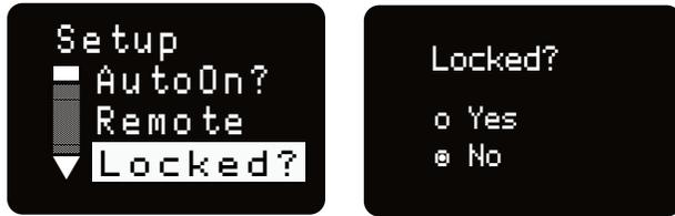
**NOTE:** If the unit is Locked, you will need to unlock it to turn the power off. This setting prevents accidentally turning off the power when in use.
