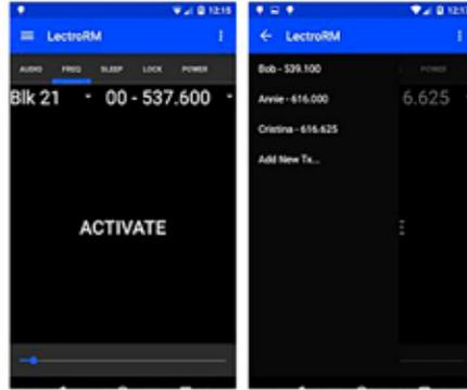
The Android version keeps all settings on the same page and allows the user to toggle between the activation buttons for each setting. The activation button must be pressed and held to activate the tone. The Android version also allows users to keep a configurable list of full sets of settings.
