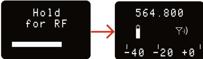
When you release the button, the unit will be operational with the RF output turned on and the Main Window displayed.
