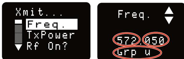
Press **MENU/SEL** and use the arrow buttons to select one of three fields to adjust: MHz, KHz and Group.
