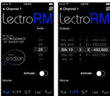
The iPhone version keeps each available setting on a separate page with the list of options for that setting. On iOS, the “Activate” toggle switch must be enabled to show the button which will then activate the tone. The iOS version’s default orientation is upside-down but can be configured to orient right-side up. The purpose for this is to orient the phone’s speaker, which is at the bottom of the device, closer to the transmitter microphone.
