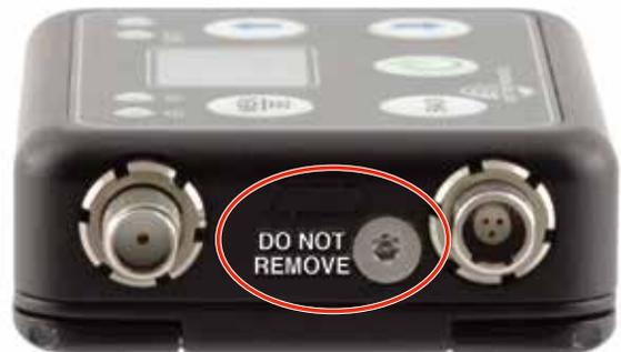
**CAUTION: DO NOT REMOVE** the threaded screw where indicated, as that will void the warranty and IP rating.
