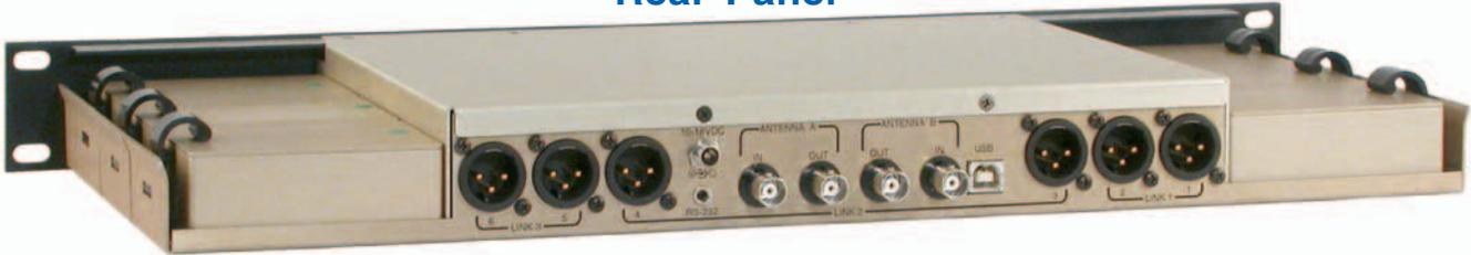
The rear panel provides six balanced audio outputs on standard XLR connectors, 50 ohm BNC antenna inputs, 50 ohm BNC antenna outputs from the built in zero-gain multicoupler, power jack with a locking connector, USB port and RS-232 serial port for the computer interface.
