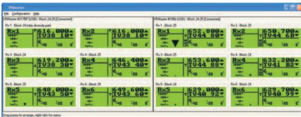
This VR Main Screen illustrates how two independent VR systems with six receivers each can be easily monitored at the same time..
