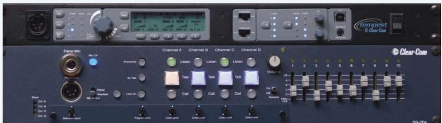
Tempest2400 Wireless Intercom System with Clear-Com Switchboard Main Station
