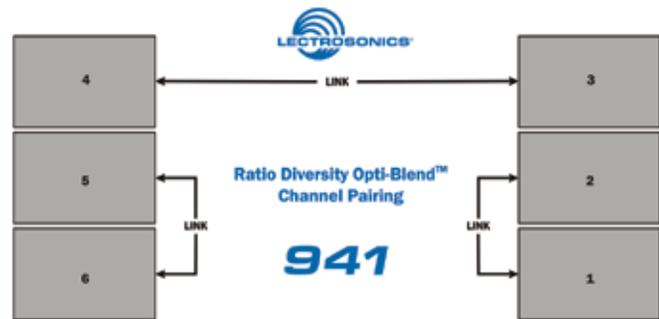
Ratio diversity employs a panning action that blends the RF signals from the two receivers over a fairly wide range of levels to eliminate dropouts before they occur. The process is called OptiBlend™ as indicated on the label on the receiver chassis.
