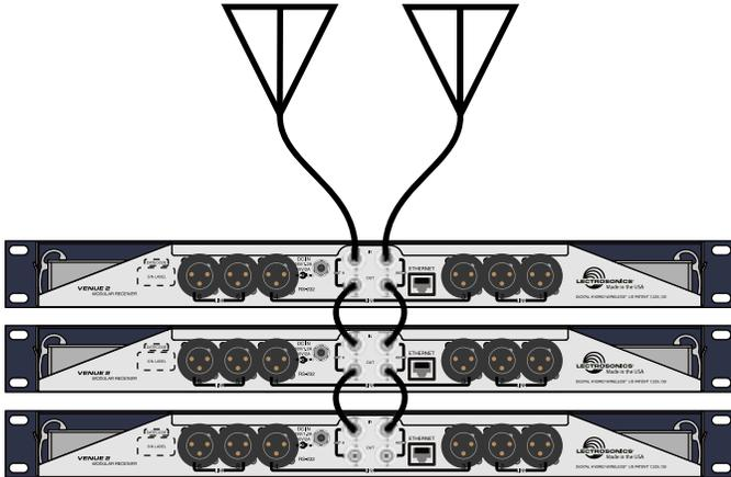
The built-in multi-coupler includes "loop through" outputs for stacking multiple Venue receivers.
