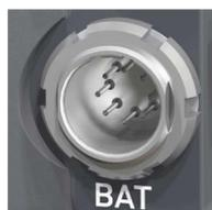
Use the BAT connector, and a KC50-S or KC50-SP-S cable, to supply the camera with 10.5 to 34 V DC.
