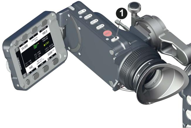
1. To change the monitor mode between live view and user interface: Press *M* (1).
