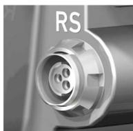
This 3-pin Fischer socket for RS input supplies external accessories with 24 V power (2.0 A). It also carries a frame pulse output and accepts an ARRI remote start/stop trigger.
