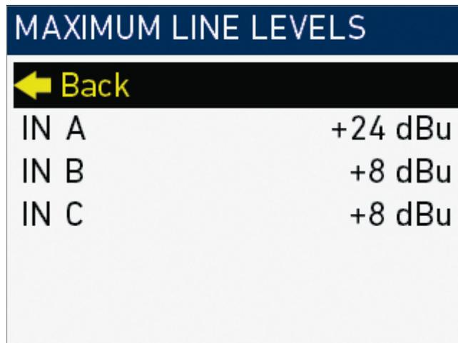
Switches the maximum line level for input A, B and C between +8 and +24 dBu.
