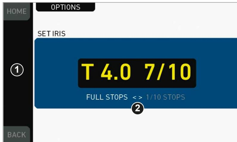
Pressing the wheel (1) changes the step size between full and sub-stops (2). **Note:** Sub-stop precision depends on the lens type and is automatically set by the camera.
