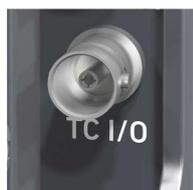
A Timecode in-/output (BNC interface) to be configured via camera menu.
