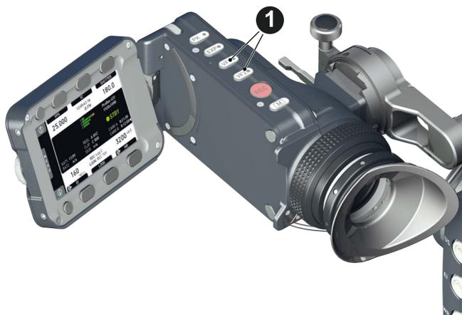
1. Via the user button menu (see "Presetting user (and VF) buttons", page 49), you can assign a function to both *VF1* and *VF2* buttons (1).
