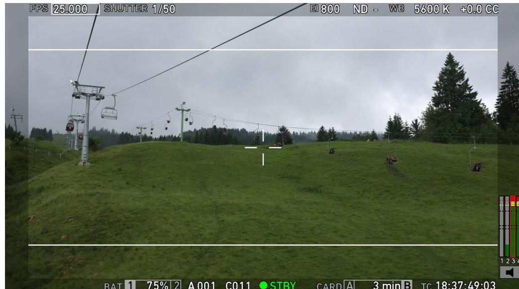
The overlay menu offers a reduced set of camera parameters for adjustment. When activated, it is visible in the top section of the image on the MVF-1 monitor and EVF and on any SDI output which has SDI processing activated. The overlay menu is a quick way to change the following camera settings:
