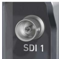
Both BNC sockets (here: SDI 1) deliver image outputs in 1920x1080 422 1.5G, 422 3G and 444 3G single link formats. SDI 2 also supports the 3840x2160 422 6G format in 4K UHD mode.
