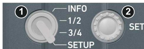
1. Turn the audio function switch to *SETUP* (1).
