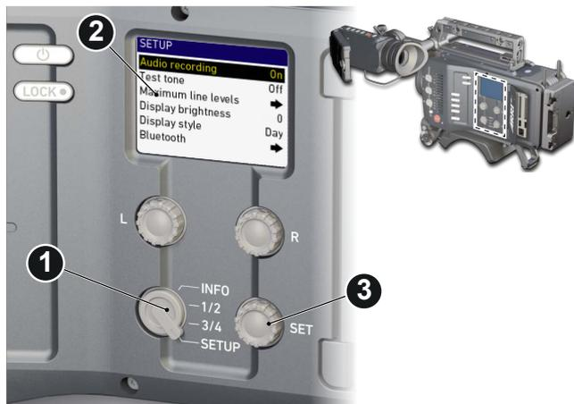
1. Select *SETUP* (1) for adjusting overall audio parameters (2).
