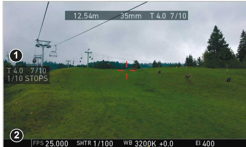
On the live screen, you can activate and deactivate iris adjustment (1) by short-pressing the lower round button (2). Keeping the button pressed (2) activates iris adjustment until it is released. (2). **Note:** Depending on the image flip, the round buttons may appear on the right.
