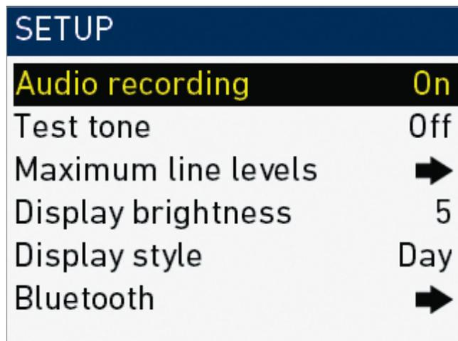
*Audio recording*: Switches audio recording on or off. *Off* deactivates audio inputs and all outputs; no audio channels are recorded.
