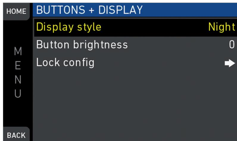
*Button brightness:* Sets the brightness of the button illumination in a range of 0 to 3.
