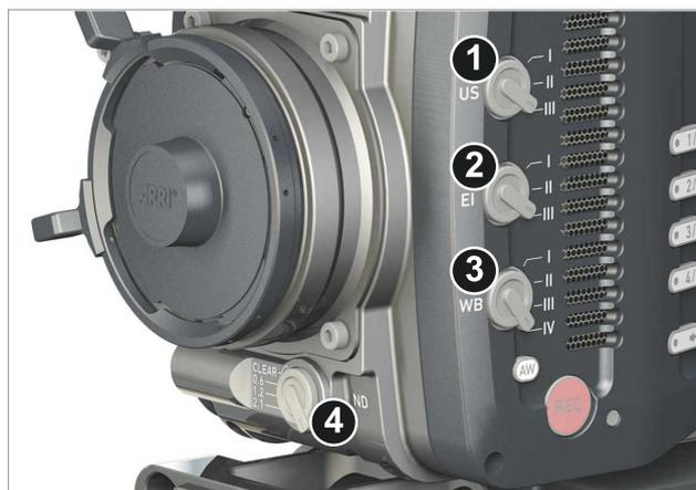
The *EI* switch (2) is dedicated to exposure index. *WB* (3) is dedicated to white balance and *ND* (4) to filtering.
