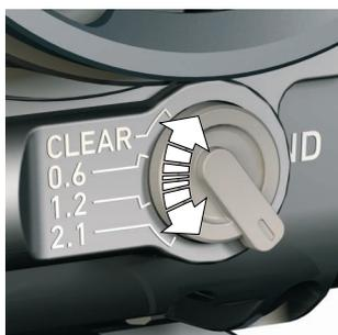
The ND filter switch controls the internal ND filter module. Filter densities of 0.6, 1.2 and 2.1 allow quick exposure changes and compensation over a range of seven stops.
