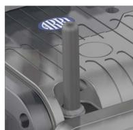
Antenna for Bluetooth signal. Used for wireless audio monitoring and comment channel return with Bluetooth headset. Supports Handsfree and A2DP protocols.
