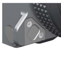
The infrared proximity sensor automatically deactivates the viewfinder's internal OLED panel when you withdraw your eye. The sensor is placed either on the bottom left-hand side of the viewfinder (generation 1, shown in image), or it is integrated into the eye cup (generation 2, not shown).
