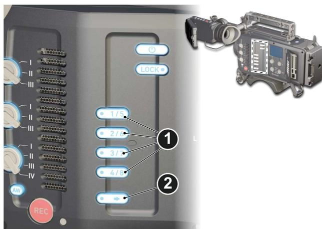
1. Press a button (1) to trigger its function.
