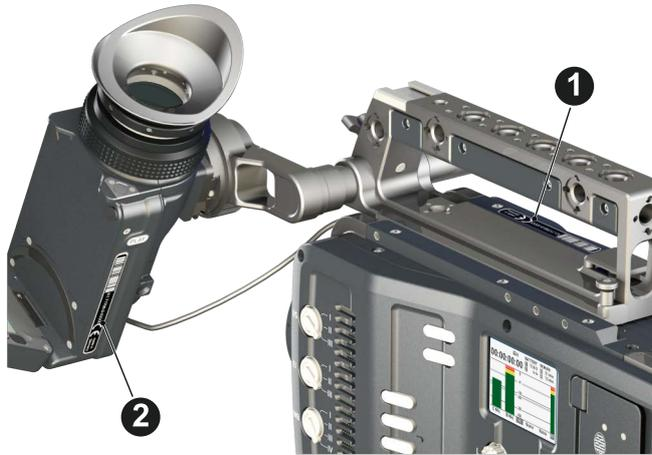
CE type labels with serial number are on the camera top (1) and under the viewfinder (2). The serial number consists of the last 5 digits of the equipment number K1.71700.0-XXXXX. An FCC conformity label is on the camera bottom.
