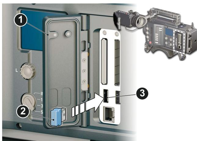
10. **For external frame files:** Store the required file(s) into *ARRI/AMIRA/FRAMELINES* on a properly prepared USB memory stick. See page 124.
